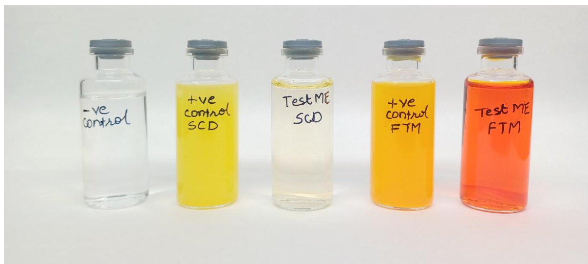
Figure 6.8: Sterility testing [A] Negative Control (Water for Injection) [B] Positive Control for Soybean casein digest medium (SCDM) [C] Test Microemulsion in SCDM [D] Positive control for Fluid Thioglycolate Medium (FTM) [E] Test Microemulsion in FTM
