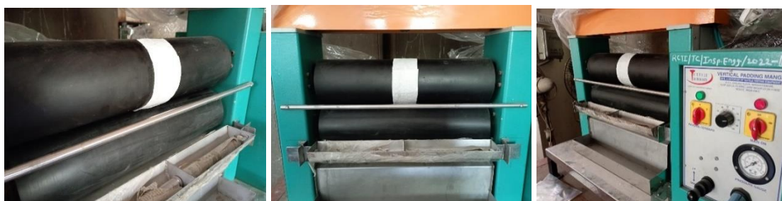
Figure 3.7: Layer-by-layer application of SAP on the top layer of sanitary napkin
