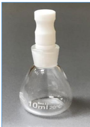
Fig. 3.14 Specific gravity bottle for density ( \rho ) measurement.
