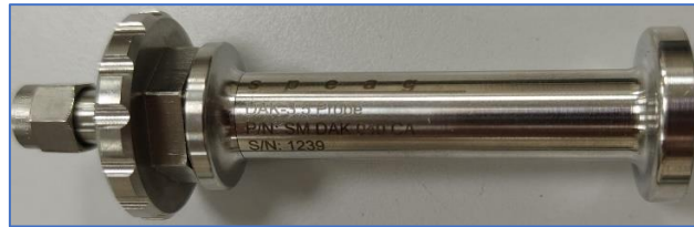
Fig. 3.6 SPEAG DAK-3.5 Probe.
