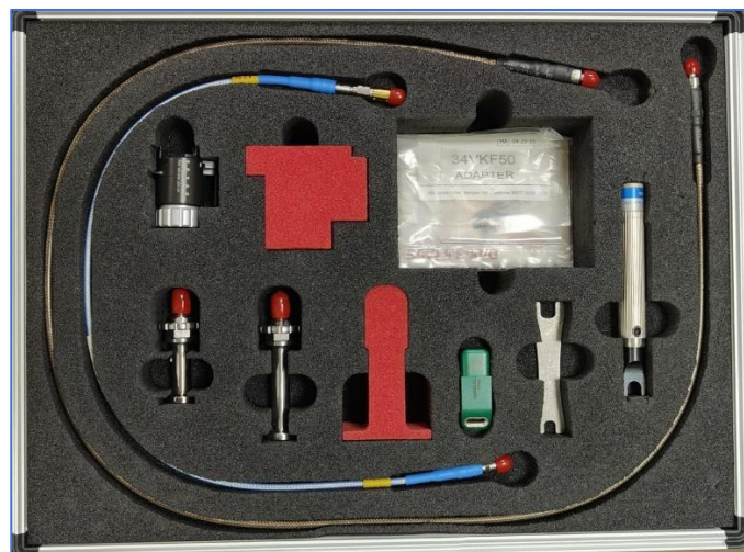
Fig. 3.7 SPEAG Dielectric Assessment Kit (DAK).
