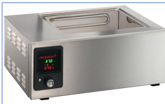
Fig. 3.2 Constant temperature water bath (Model Industrial Corporation).
