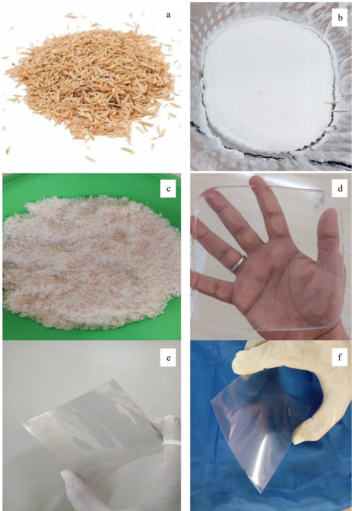
Figure 10: (a) Raw Agricultural Residues, (b) Pulp obtained after bleaching treatment, (c) Dried crystalline powder after hydrolysis, (d) Wet transparent Sheet obtained after regeneration, (e) Dried sheet cut in 10 cm x 10 cm, (f) Sheet after ITO Sputtering.
