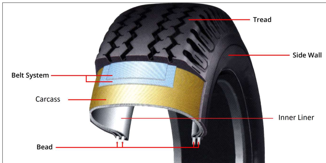
Figure-1: Different part of a tyre
