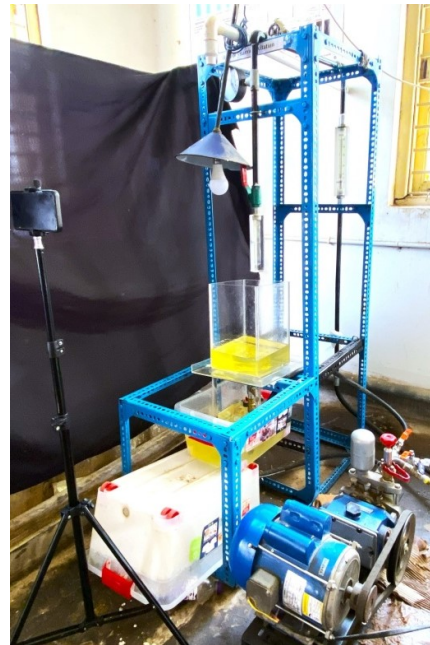
Fig 13 (b) Actual image of the experimental test facility to visualize the cavitation flow
