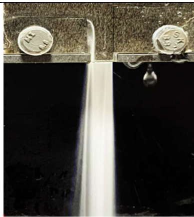
Water, P_{inj} = 4.9 bar, \theta = 7^\circ
