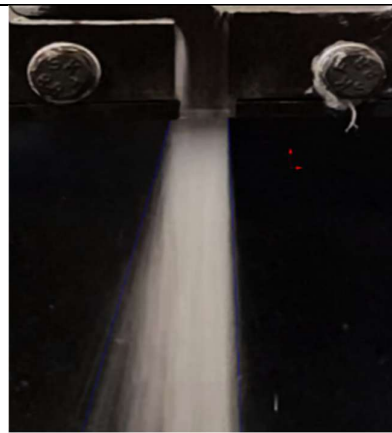
Diesel, P_{inj} = 6.6 bar, \theta = 11^\circ
