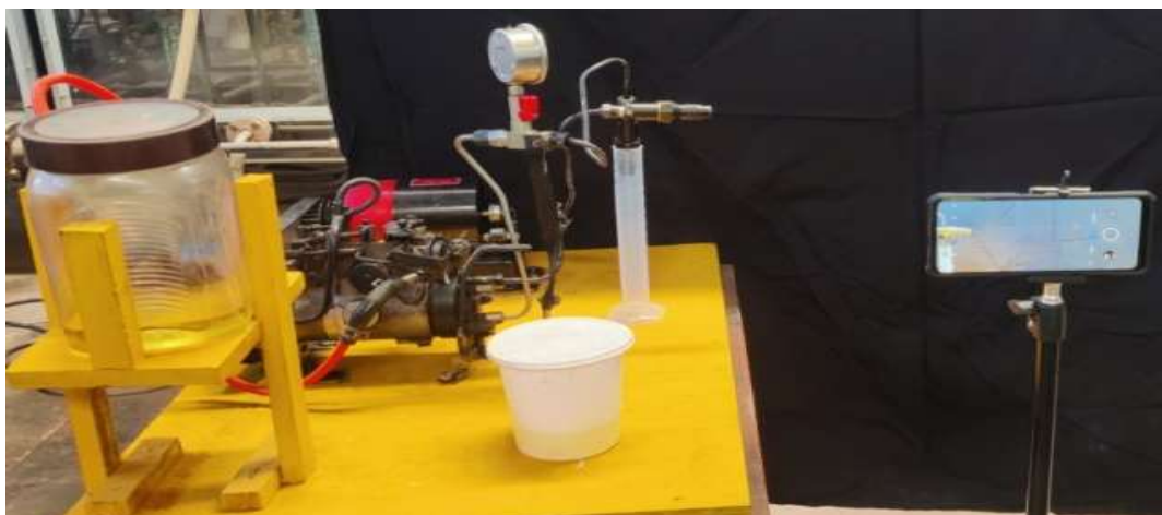
Fig. 3.13 Actual image of test set up to visualization of spray characteristics
