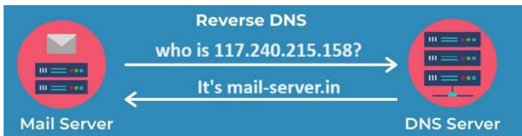
Figure 21: Reverse DNS process flow
