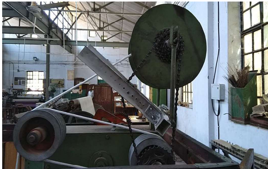
Figure 3.5 Take up zone for braiding machine
