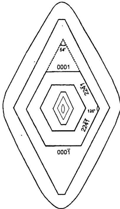
**Figure 4.1** : Illustrating formation of apparent hexagonal looking growth features on prism faces of beryl crystal, due to the development of 0001 (basal pinacoid) and 2241 (dipyramid of 2<sup>nd</sup> order) faces.
