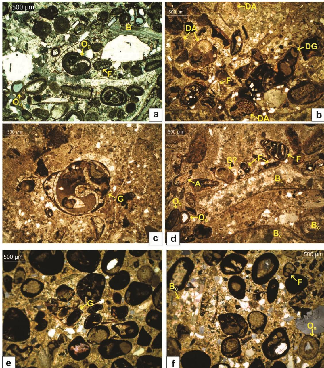
**Plate 4.15** Photomicrographs of oolitic packstone microfacies shows the compositional variations.
