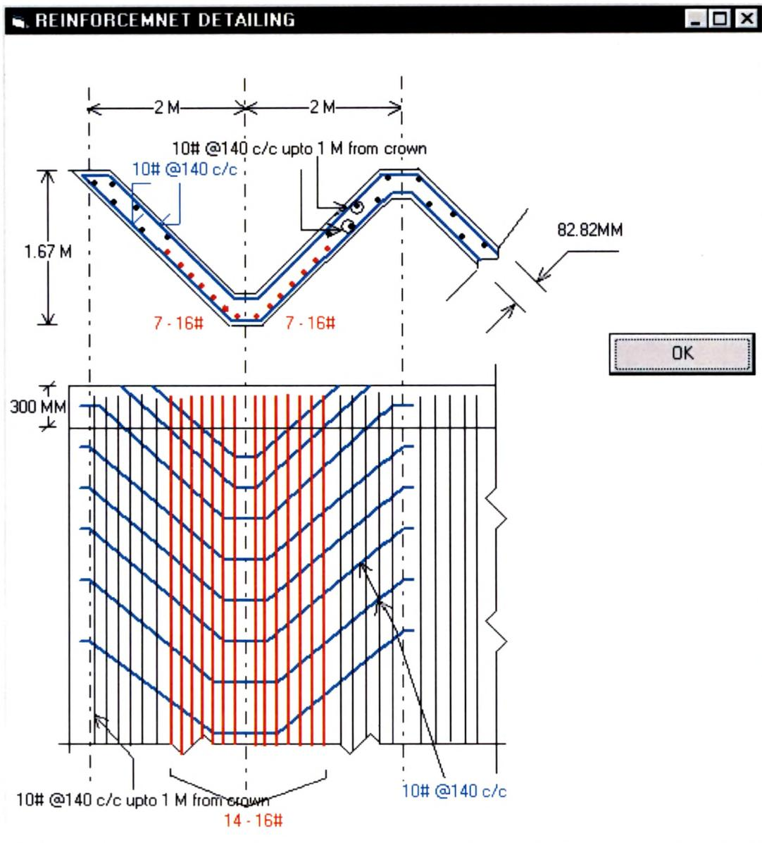
**Fig. 8.34 Form Showing Detailing of the folded Plate Section**
