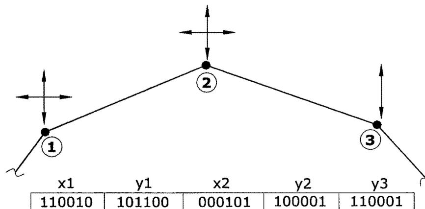
**Fig. 8.53 Representation of Configuration Variables**
