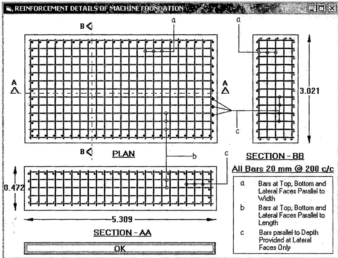
Fig. 8.44 Reinforcement Detailing for Machine Foundation
