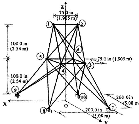
**Fig. 8.82 Geometry of 25 bar Space Truss**
