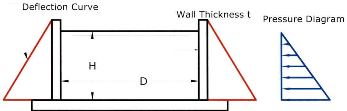
**Fig 8.4 Deflection Curve and Pressure Distribution on Tank**
