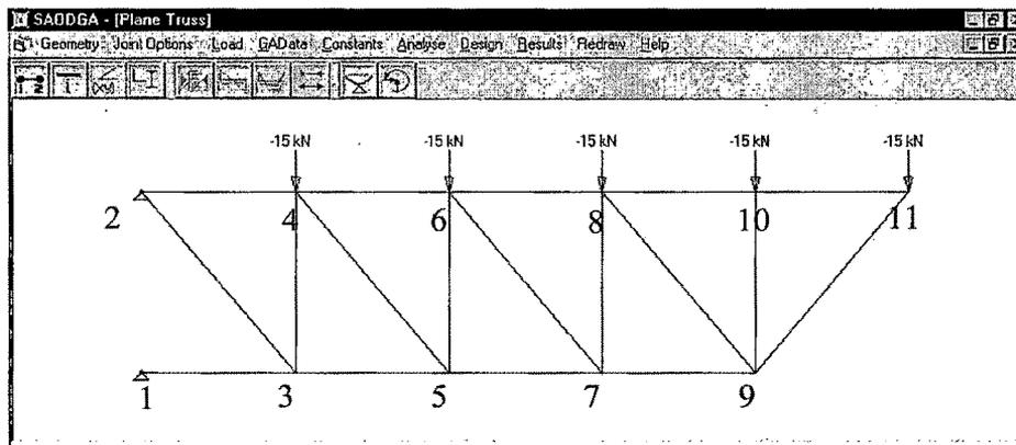
**Fig. 8.67 Initial Geometry with Support and Loading Condition**
