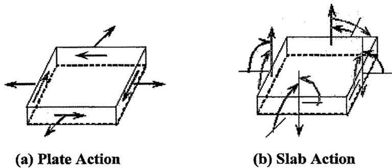
**Fig. 8.30 Elements of Folded Plates under Different Actions**
