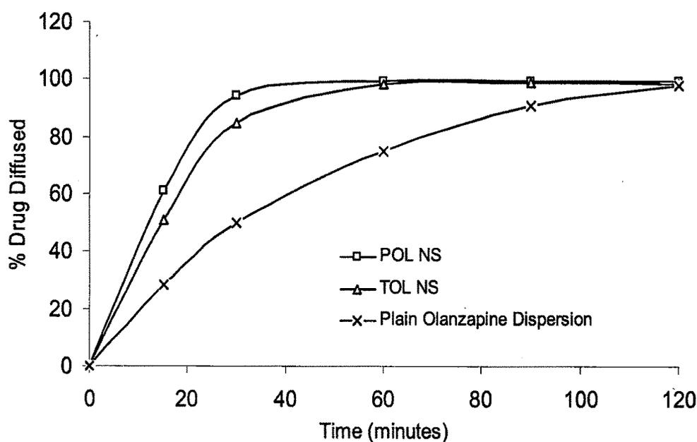
**FIGURE 10.5: In vitro diffusion of OL from the OL solution and OL nanosuspension in phosphate buffer pH 7.4**
