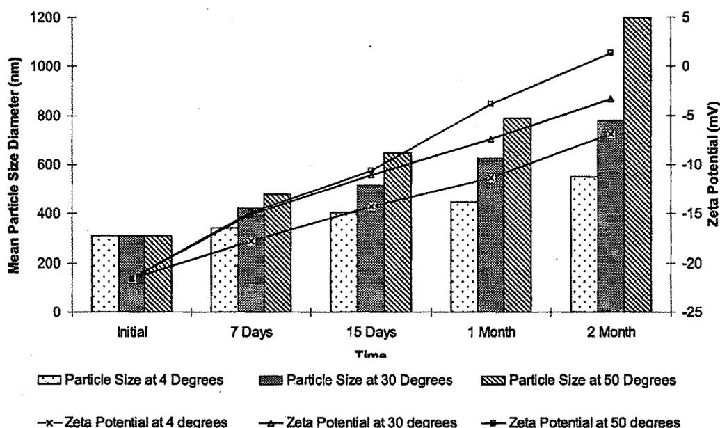
**FIGURE 10.7: Mean particle Diameter and zeta potential of TOL NS dispersion stored at different temperatures in dark condition.**
