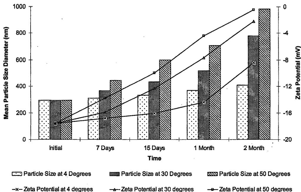
**FIGURE 10.6: Mean particle Diameter and zeta potential of POL NS dispersion stored at different temperatures in dark condition.**
