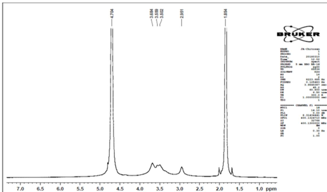
**Figure 4.6:** <sup>1</sup>H-NMR spectrum of Trimethylated Chitosan-4(TMC-4)
