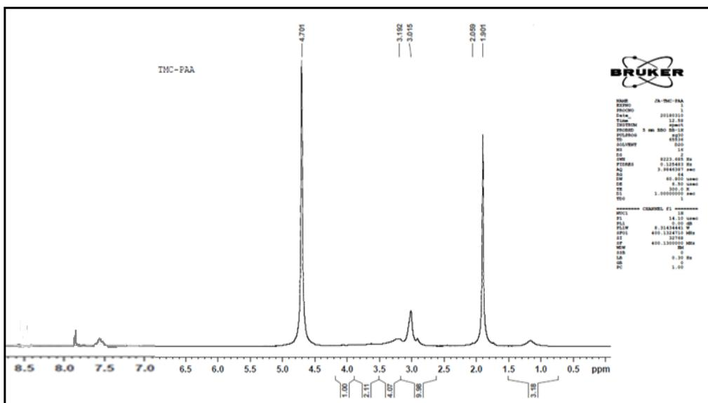
Figure 4.15:  $^1\text{H}$ -NMR spectrum of the 3-Pyridyl acetic acid conjugated TMC 31
