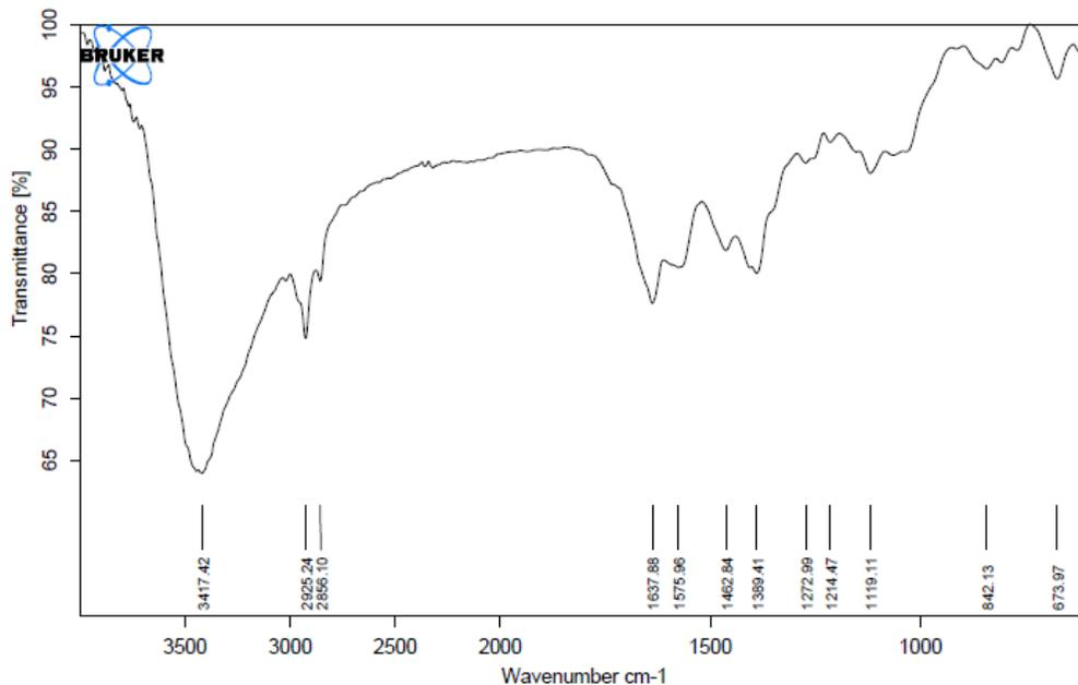
**Figure 4.18: FTIR spectrum of 3-Pyridyl acetic acid conjugated TMC 31**
