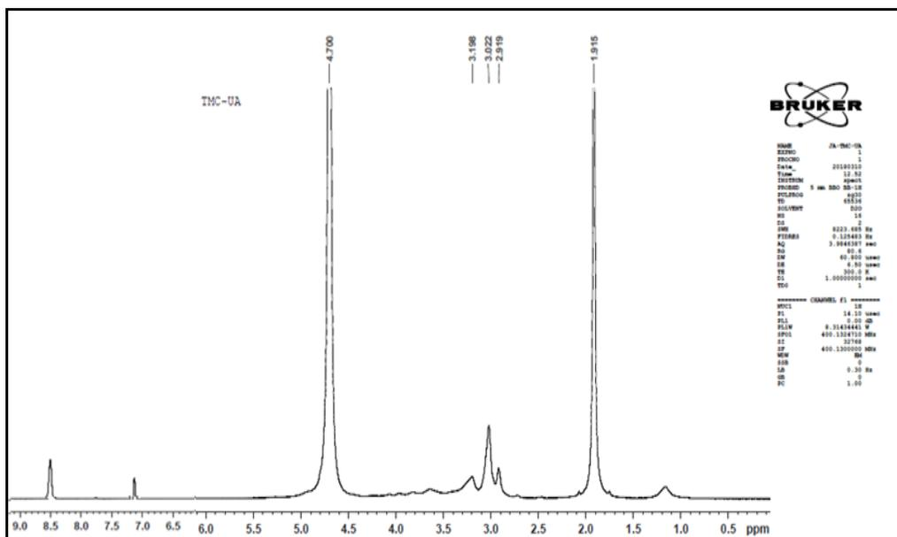
Figure 4.13:  $^1\text{H-NMR}$  spectrum of the Urocanic acid conjugated TMC 31
