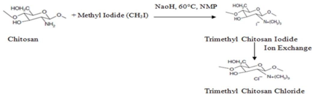
**Figure 4.1: Synthesis steps of N,N,N-Trimethylated chitosan**
