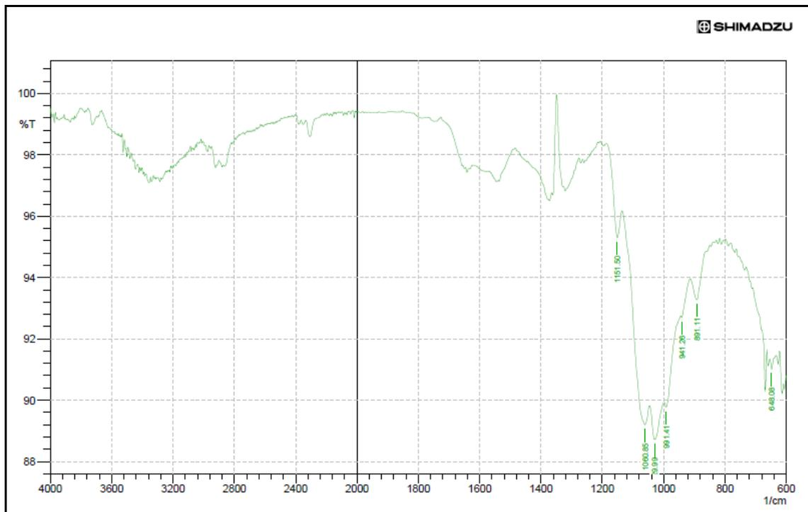
**Figure 4.9: FTIR spectrum of Chitosan**
