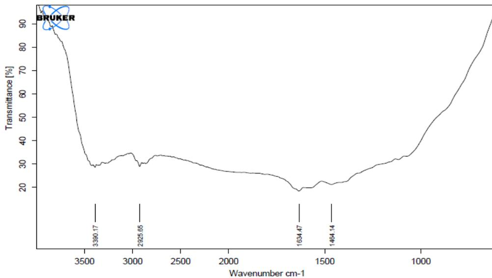
Figure 4.17: FTIR spectrum of Piperazine 2-Carboxylic acid conjugated TMC 31
