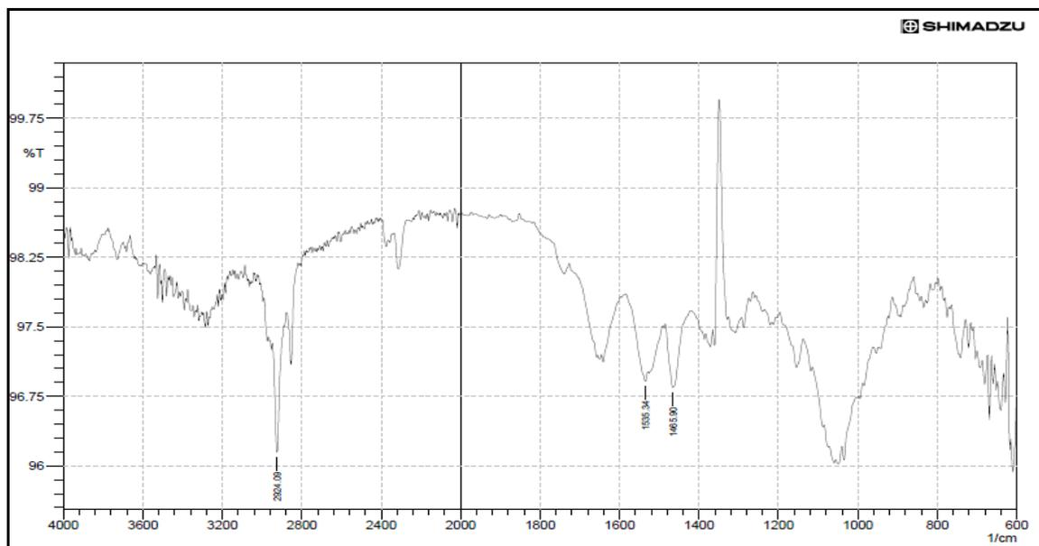
Figure 4.7: FTIR spectrum of Trimethylated Chitosan-1
