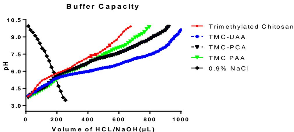
**Figure 4.20: Acid/Base titration of different modified TMCs**
