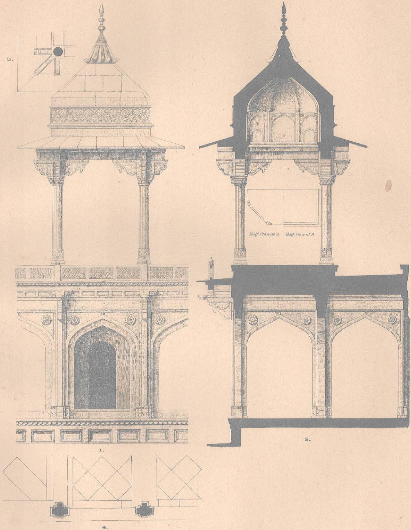
ELEVATION AND DETAILS OF A BAY: SECOND FLOOR.
